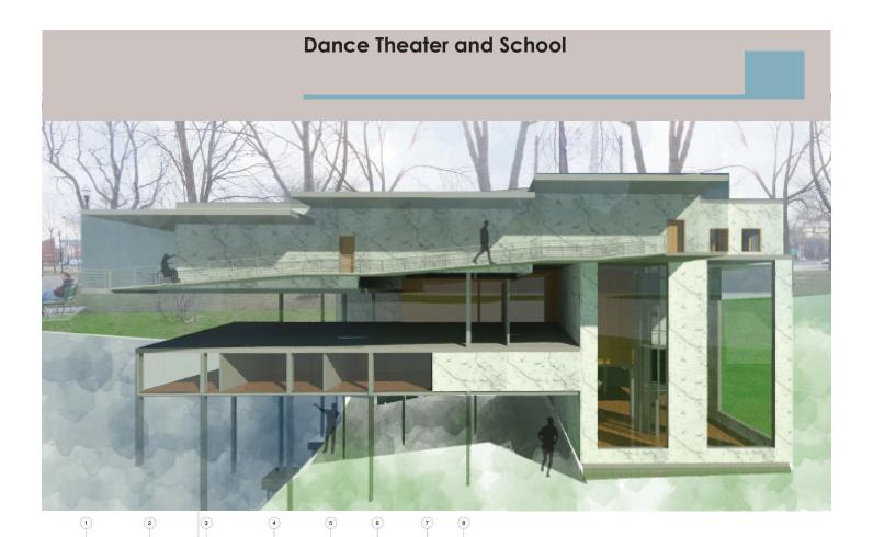
Due to its close proximity to the river, the ground floor of the building has a small footprint on higher ground farthest from the river's edge. In addition to mitigating the effects of sea level rise, raising the majority of the building mass allows users of the park pathway to walk under the building, creating a link between the it and the site at the human scale.
