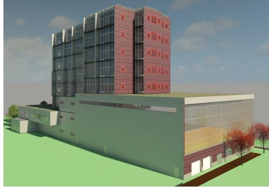
Brick cladding was for chosen the building envelope to fit in with the character of the Pine Street Inn's historic building and warehouses nearby. Curtain wall and channel glass were used to tie in with the new construction, also nearby, as well as provide maximum daylight.
