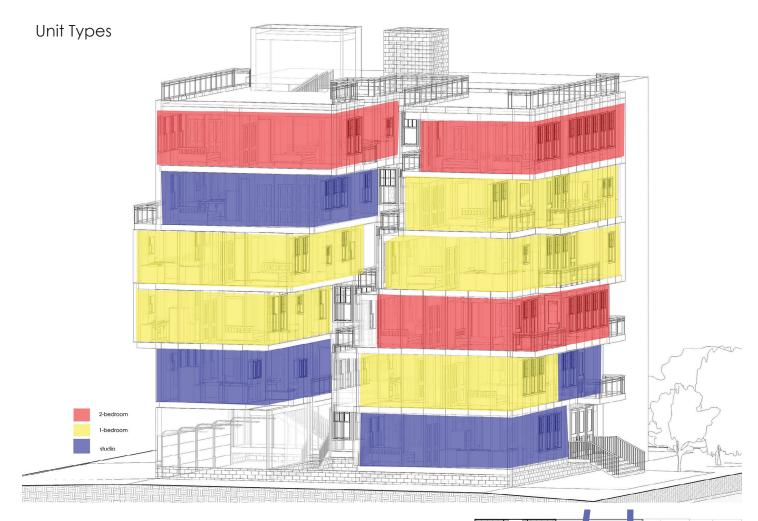
Since the height was restricted to 65 feet, the floor-to-floor height was limited to 10 feet to maximize the number of units. The finished project consisted of four studios, six one-bedroom and three two-bedroom units ranging from 300 to 897 square feet.
